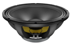
No. 12602539 LAVOCE SAF184.01 18" Subwoofer Ferrite Magnet Aluminium Basket Driver 700 W AES, 8 ohms, 99 dB, 30-1500 Hz
