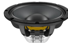
No. 12602612 LAVOCE WAN082.00 8" Woofer Neodymium Magnet Aluminium Basket Driver 200 W AES, 8 ohms, 95.5 dB, 75-3000 Hz
