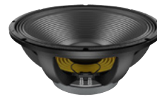
No. 12602540 LAVOCE SAF184.02 18" Subwoofer Ferrite Magnet Aluminium Basket Driver 1200 W AES, 8 ohms, 97 dB, 40-1000 Hz
