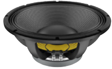
No. 12602535 LAVOCE WAF154.02 15" Subwoofer Ferrite Magnet Aluminium Basket Driver 800 W AES, 8 ohms, 96 dB, 40-1000 Hz
