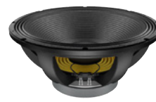
No. 12602542 LAVOCE SAF184.04 18" Subwoofer Ferrite Magnet Aluminium Basket Driver 1500 W AES, 8 ohms, 95 dB, 35-1000 Hz
