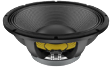
Best.-Nr. 12602535 LAVOCE WAF154.02 15" Subwoofer, Ferrit, Alukorb 800 W AES, 8 Ohm, 96 dB, 40-1000 Hz
