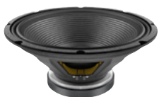
Best.-Nr. 12602538 LAVOCE SSF184.00 18" Subwoofer, Ferrit, Stahlkorb 1000 W AES, 8 Ohm, 97 dB, 30-800 Hz
