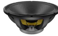
Best.-Nr. 12602541 LAVOCE SAF184.03 18" Subwoofer, Ferrit, Alukorb 1500 W AES, 8 Ohm, 96 dB, 30-1000 Hz
