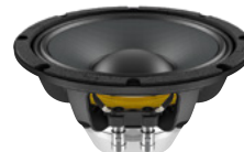
Best.-Nr. 12602612 LAVOCE WAN082.00 8" Woofer, Neodym, Alukorb 200 W AES, 8 Ohm, 95,5 dB, 75-3000 Hz
