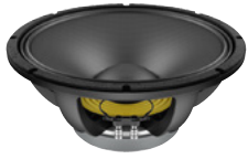
Best.-Nr. 12602534 LAVOCE WAF153.00 15" Woofer, Ferrit, Alukorb 500 W AES, 8 Ohm, 99 dB, 45-3000 Hz
