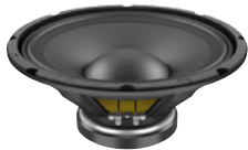
No. 12602525 LAVOCE WSF122.02 12" Woofer Ferrite Magnet Steel Basket Driver 200 W AES, 8 ohms, 97.5 dB, 50-3000 Hz
