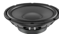
No. 12602521 LAVOCE SSF102.40 10" Subwoofer Ferrite Magnet Steel Basket Driver 250 W AES, 8 ohms, 92 dB, 40-500 Hz
