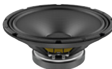
Best.-Nr. 12602519 LAVOCE WSF101.82 10" Woofer, Ferrit, Stahlkorb 150 W AES, 8 Ohm, 97,5 dB, 63-3000 Hz
