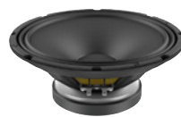
Best.-Nr. 12602520 LAVOCE WSF102.00 10" Woofer, Ferrit, Stahlkorb 175 W AES, 8 Ohm, 97 dB, 60-4000 Hz
