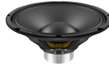
No. 12603214 LAVOCE NBASS12-30 12" Bass Guitar Woofer Neodymium Magnet Steel Basket Driver 400 W AES, 8 ohms, 98 dB, 50-3000 Hz
