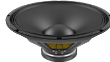
No. 12603216 LAVOCE FBASS15-20 15" Bass Guitar Woofer Ferrite Magnet Steel Basket Driver 200 W AES, 8 ohms, 98 dB, 40-4000 Hz
