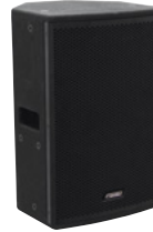
Best.-Nr. 11041100 PSSO K-210 2-Wege-Top 300W Profi-PA-Box, 10" Woofer, 1" Horn, 300 W RMS, 8 Ohm
