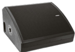
Best.-Nr. 11041119 PSSO K-215CM 2-Wege-Koaxial-Monitor 400W Profi-PA-Box, 15" Woofer, 1,4" Horn, 400 W RMS / 8 Ohm
