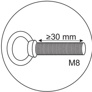
**Please note:** the speaker-system must always be secured via three appropriate eye-bolts and three appropriate safety bonds.
