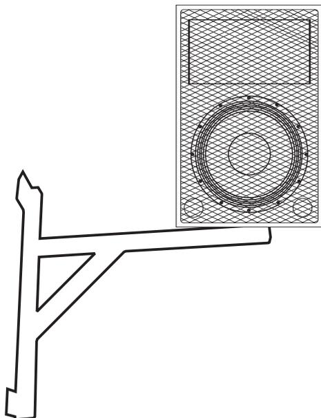
The speaker-system may only be installed on a wall-mounting if the original speaker-system is equipped with an appropriate flange.
