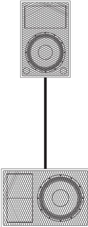
A satellite-system is a system where a speaker-system with flange is installed on top of a subwoofer.
