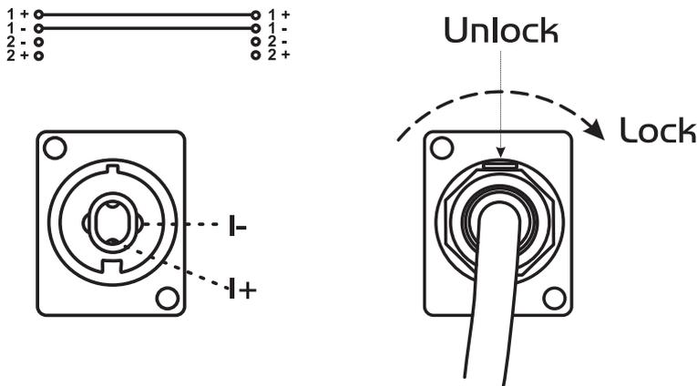
**Installing the speaker-cables**
