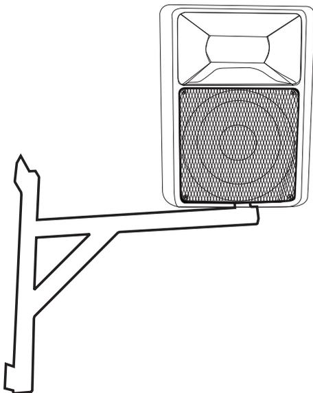
Before attaching the speaker-system, make sure that the installation area can hold a minimum point load of 10 times the installation's weight (e.g. 13 kg weight - 130 kg point load).
