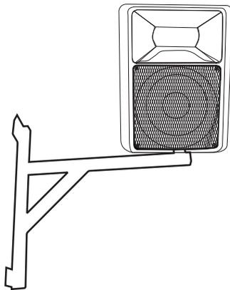
Before attaching the speaker system, make sure that the installation area can hold a minimum point load of 5 times the speaker system's weight.
