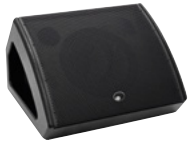
No. 11038038 OMNITRONIC KM-110 Stage Monitor, coaxial Monitor with 10" woofer, 1.35" driver and 200 W RMS / 8 ohms
