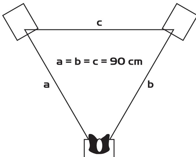
Install your monitors in an isosceles triangle where the distances between the speakers and the listener are the same ( $a = b = c = \text{ca. } 90 \text{ cm}$ ).
