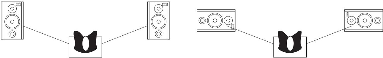
These monitors are magnetically shielded so that you can install them next to monitors, e.g. computers or video processing devices. Nevertheless keep a minimum distance of 8 cm to the monitor. If the image of a sensitive device is distorted nevertheless, increase the distance.
