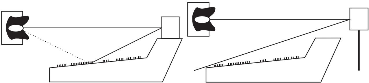
Do not direct the monitors in front, but rather rotate them slightly towards the listener. In order to avoid reflections from the ceiling or floor, the tweeters should be located as high as your ears.
