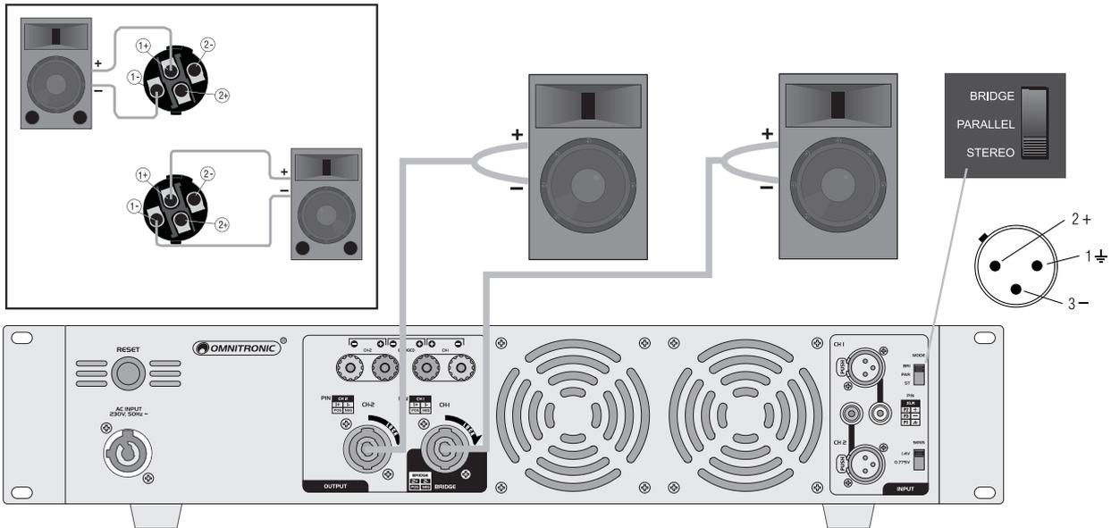
**Fig. 1** Stereo wiring using the speaker connectors
