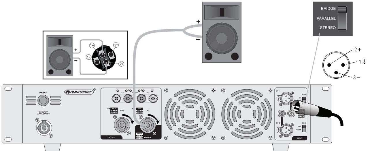
Fig. 5 Bridge wiring using the speaker connectors
