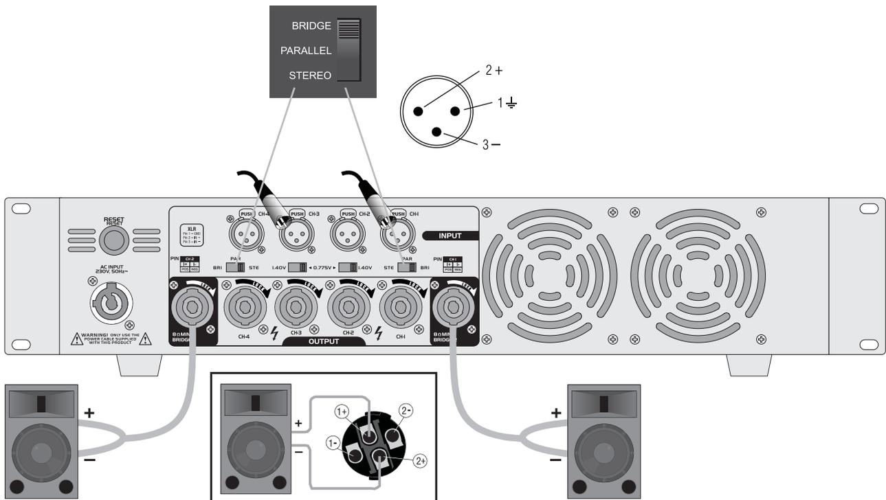
Fig. 9 Wiring in bridge mode
