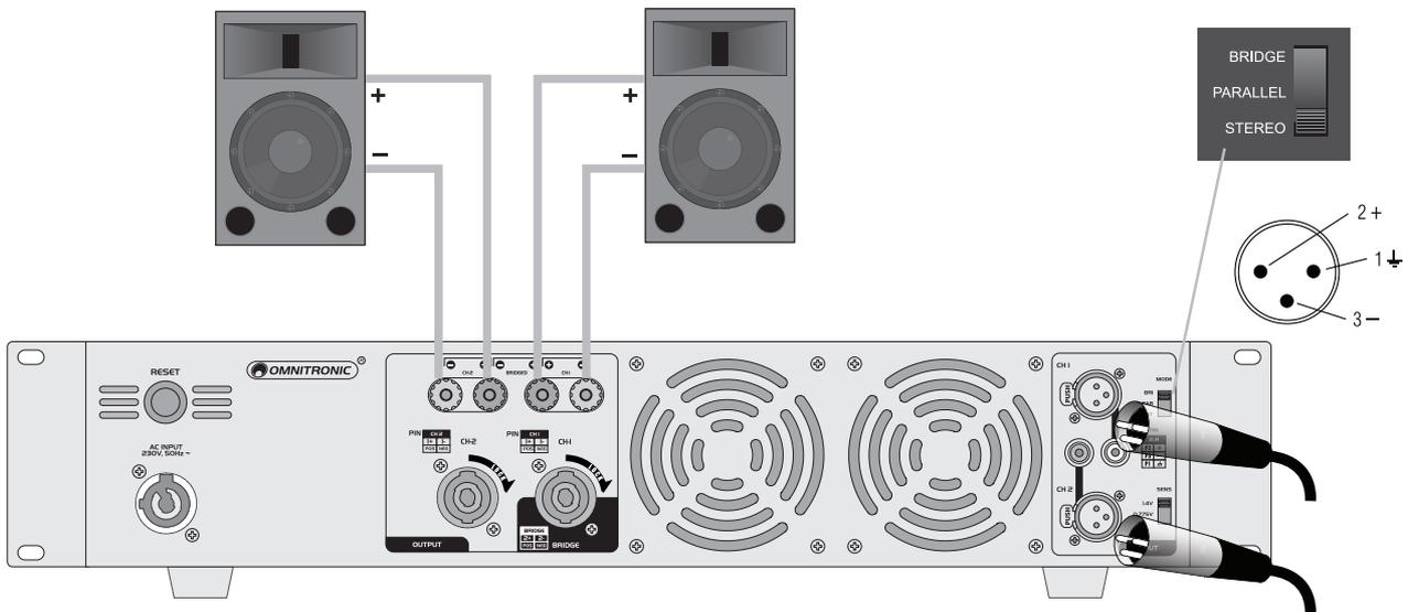
**Fig. 2** Stereo wiring using the screw terminals
