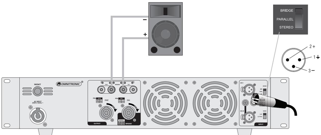
Fig. 6 Bridge wiring using the screw terminals
