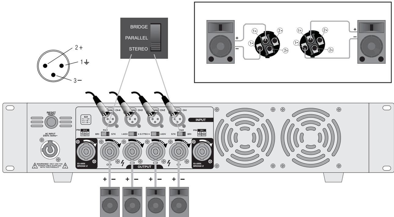
Fig. 7 Wiring in stereo mode
