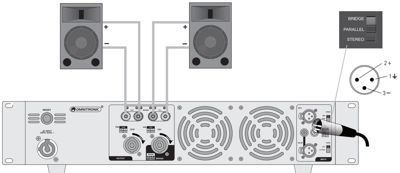
Fig. 4 Parallel wiring using the screw terminals
