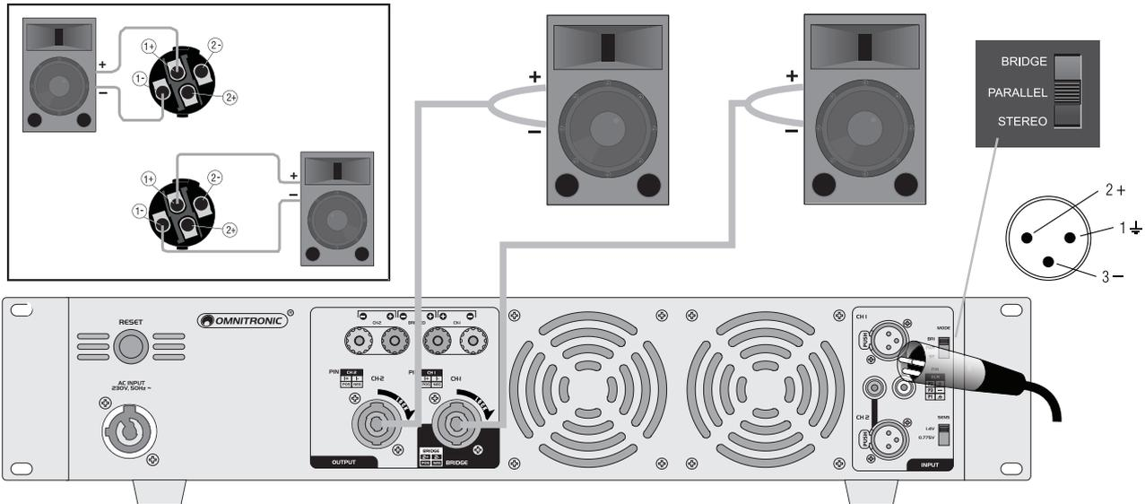
Fig. 3 Parallel wiring using the speaker connectors
