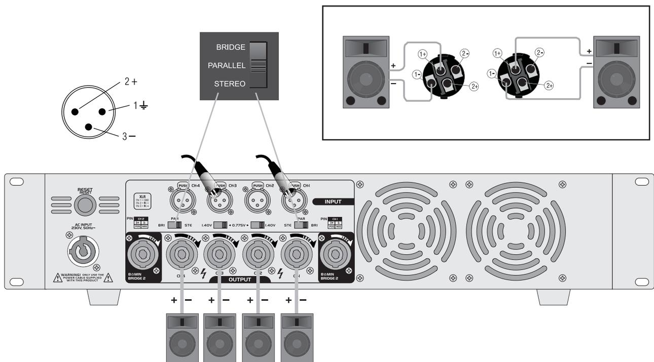
Fig. 8 Wiring in parallel mode
