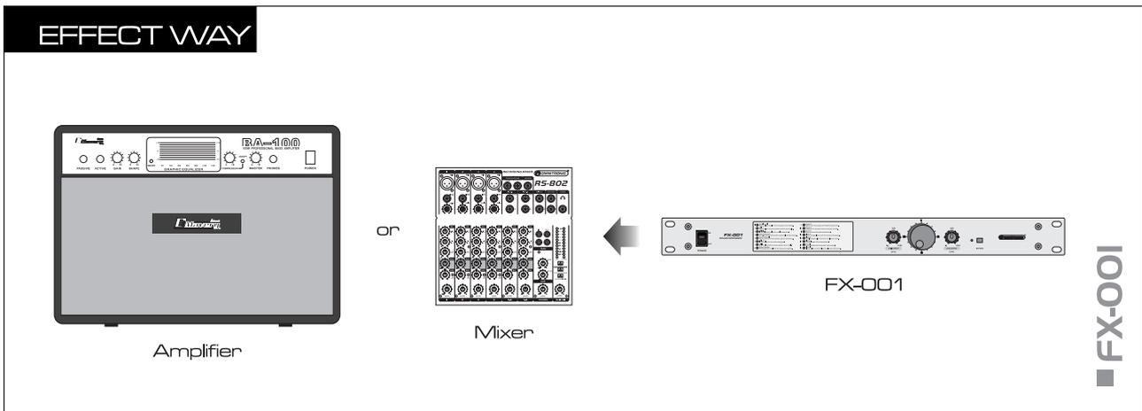
The FX-001 can be inserted via the inputs and outputs into the effect way of a mixer or instrument amplifier.
