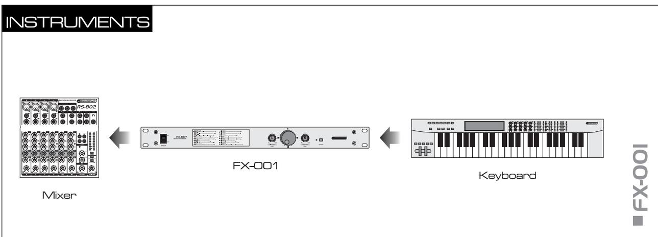
The FX-001 can also be inserted between two units (e.g. as effect unit for stage instruments).
