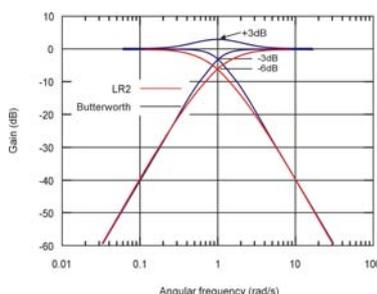
When using Linkwitz-Riley filters, the upper and lower crossover frequency of consecutive frequency bands can have the same frequency. The mostly available Bessel filters have a less strong bended amplitude compared with Butterworth filters, but a better frequency response and constant group delays. Common abbreviations for Butterworth is BW, for Linkwitz-Riley L-R (not to be mixed up with left/right).
