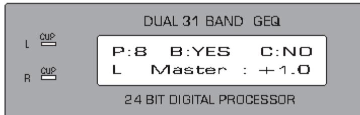
Adjust the desired program by turning the Jog-wheel. Confirm with button B or cancel with button C.
