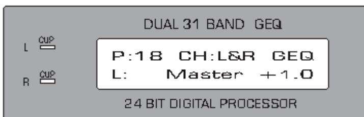
Press the Frequency-button and adjust the desired frequency (between 20 Hz and 20 kHz) via the Jog-wheel. Press the Frequency-button again and adjust the Gain-level via the Jog-wheel. Press the Frequency-button again to memorize the settings.
