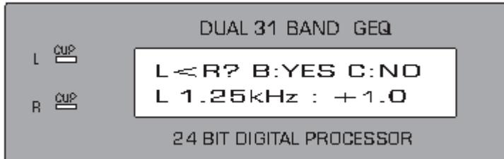
With the copy-function, you can copy the settings of one channel to the other. Press the Edit-button and check the copying direction. Confirm with button B or cancel with button C.
