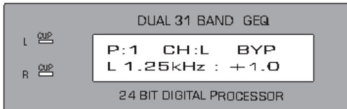
Press the Bypass-button. The display shows „BYP“ and the equalizer is bypassed. Press the Bypass-button again and the display shows „GEQ“. The equalizer is active again.
