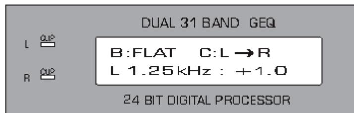
Press the Edit-button. Press the button B in order to enter Flat-mode. All frequencies have been set to 0 dB.
