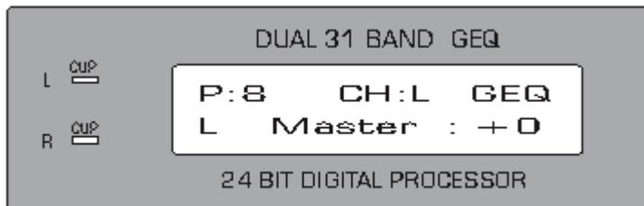
Via the button CH-SEL, you can adjust the desired channel, mono „L“ or „R“. For adjusting stereo „L & R“ hold the Edit-button until the display shows „L & R“.
