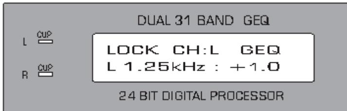
Hold the Lock-button until the display shows „LOCK“. All functions (including the jog-wheel) are locked. In order to reset, hold the Lock-button until „LOCK“ disappears from the display.
