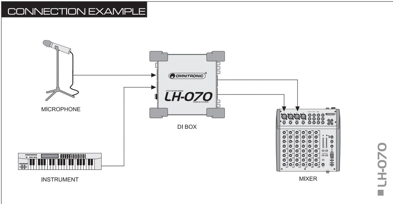
1. Connect the outputs of your musical instruments (balanced or unbalanced) via XLR plugs to the inputs 1 and 2.
