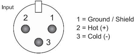
For unbalanced use pin 1 and pin 3 have to be bridged
