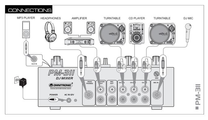
Switch off the mixer prior to connecting any units or to changing any existing connections.
