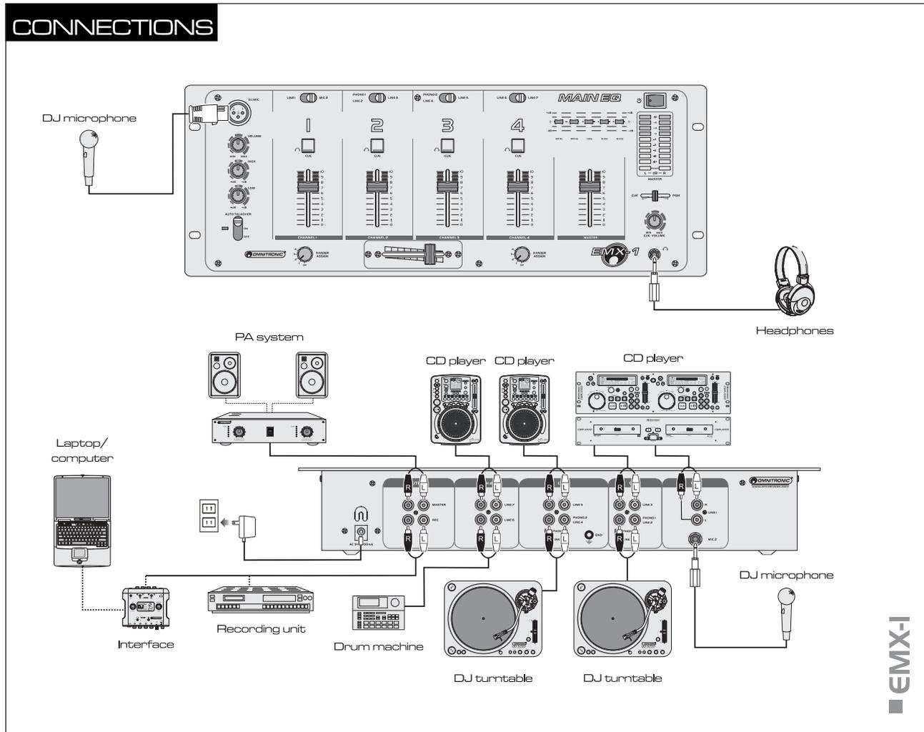
Switch off the mixer prior to connecting any units or to changing any existing connections.
